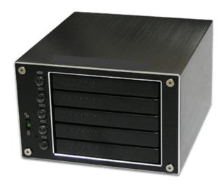
The Wrangler DataCube is fully OS independent. It can be connected to any computer running Windows, Linux or Mac OS. The power and the small size of the DataCube makes it an ideal high performance RAID storage solution for moving video data from location to editorial.
